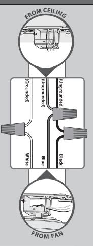
Turn the splices upward and push them carefully back through the hanger bracket into the outlet box. Spread the wires apart, with the grounded wires on one side of the outlet box and the ungrounded wires on the other side of the outlet box.
